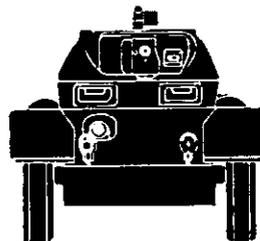
**INTEREST DATA:** This car is built in the United States for the British. It has been given the name "Staghound." The vehicle is classed as a medium armored car. It is equipped with a smoke projector on the right side of the turret roof.
