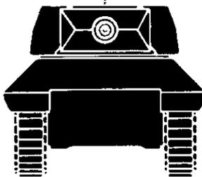
**INTEREST DATA:** This vehicle mounts a 3-inch gun in a turret on a modified M3 medium tank chassis. It has been the standard tank destroyer weapon, but is being replaced by the T70. It performed well in North Africa, where it was of great assistance in stopping German tank attacks.
