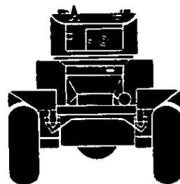
**INTEREST DATA:** This vehicle is called the "Matador." Latest models mount a 6-pounder. The vehicle is not fast, but is very reliable and can negotiate heavy sand and mud, and has been used principally in the Middle East.
