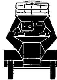
**INTEREST DATA:** The body of this vehicle is very similar to that of the German 8-wheeled armored car. The four rear wheels are powered, and the vehicle may be driven in either direction. Two versions of this vehicle are designated Sd Kfz 231 and 263.
