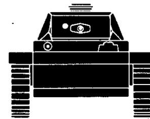
**INTEREST DATA:** Early models of this tank were very lightly armored. Protection of the vehicle has been improved gradually by the use of better and thicker armor plate; also in the later models provision is made for attachment of additional armor. Armament has also been made more powerful, the tank having first a short 50-mm gun, then a long 50-mm gun, and more recently short and long 75-mm guns. The chassis has also been used as a self-propelled mount for 75-mm assault guns.
