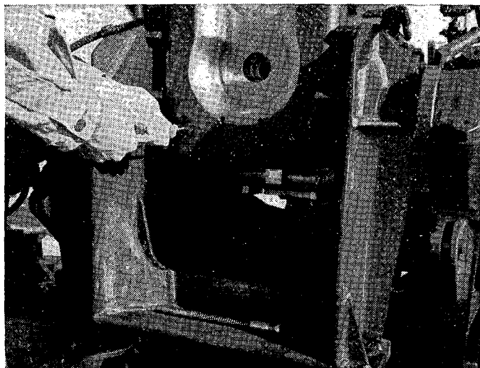
FIGURE 11.—Removal of breechblock.
