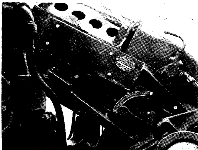
FIGURE 15.—Left side of gun, showing vent plug, recoil cylinder plug, breech operating cam lever, and control bar.
