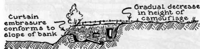
FIGURE 188.—75-mm gun in bank along edge of road.
