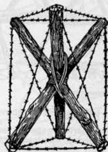
FIGURE 169.—Hedgehog (used to block trenches).
