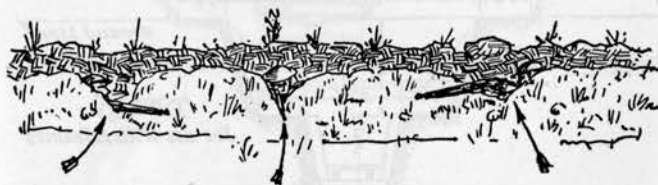
FIGURE 125.—Trench with irregular parapet and parados.
