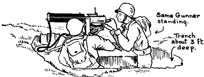
FIGURE 31.—Standing type heavy machine-gun emplacement.
