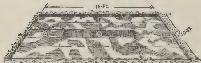
FIGURE 8.—Flyproofing latrine pit. A—Oil soaked burlap extending completely around pit. B—Opening of pit. C—Sidewall of excavation in which burlap is placed.
