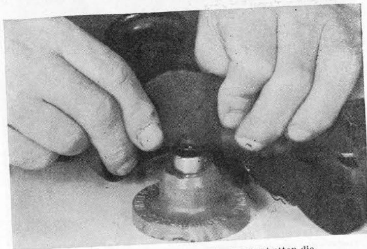
FIGURE 78.—Placing new rivet button on button die.
