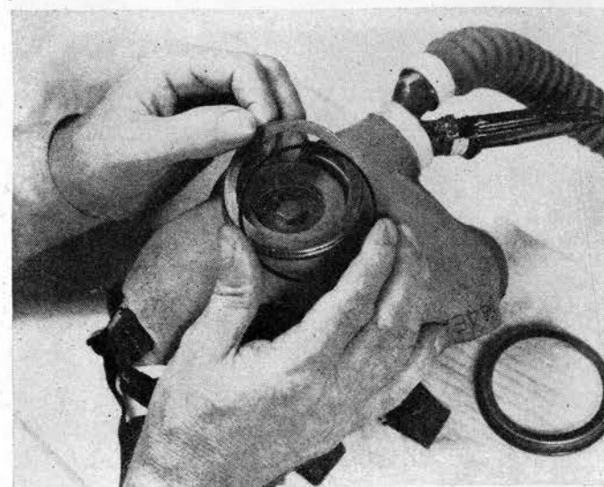
FIGURE 55.—Inserting new gasket and lens.
