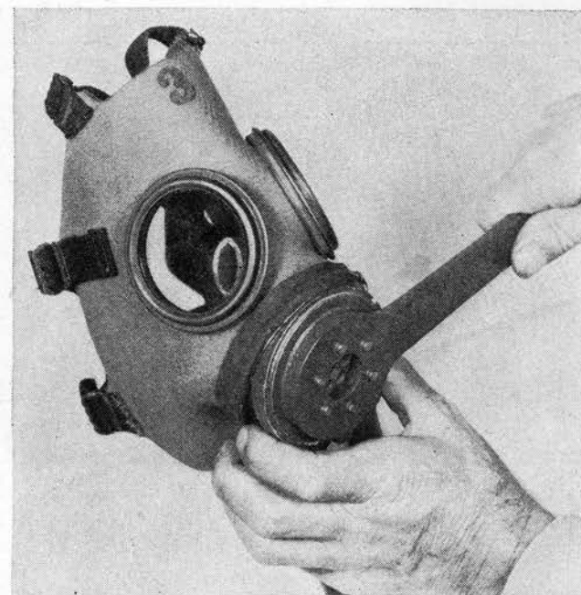
FIGURE 52.—Replacing diaphragm in MI diaphragm assembly using combination wrench (item 5).
