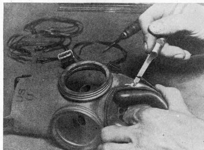
FIGURE 67.—Tightening wire clamp—MII diaphragm mask.
