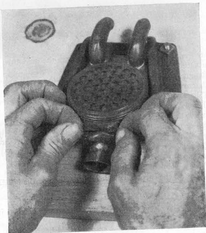
FIGURE 54.—Replacing outlet valve on MII diaphragm angletube.
