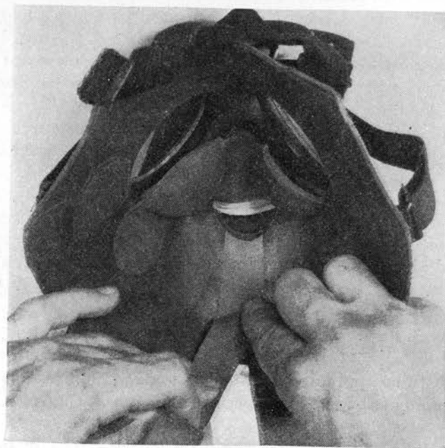
FIGURE 44.—Applying chin seam tape.
