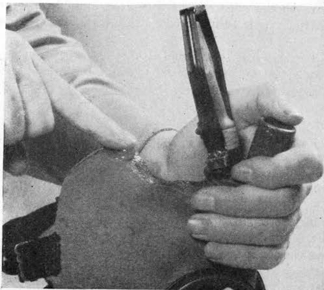
FIGURE 43.—Applying rubber cement to chin seam.
