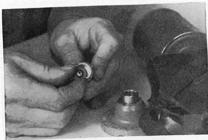
FIGURE 81.—Placing washer in handchuck.
