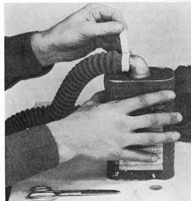
FIGURE 62.—Placing tape around wire.
