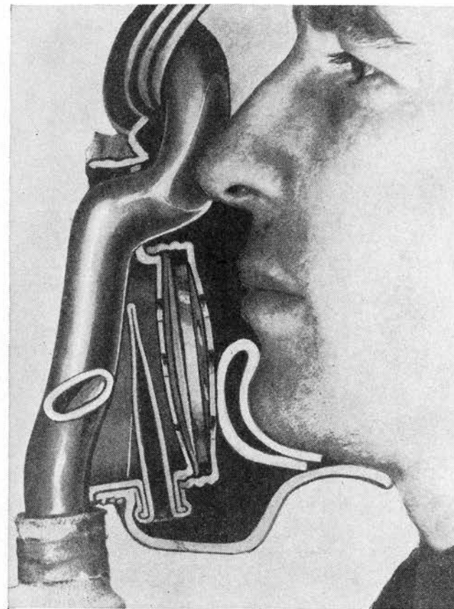
FIGURE 11.— MII diaphragm angletube, sectional view.
