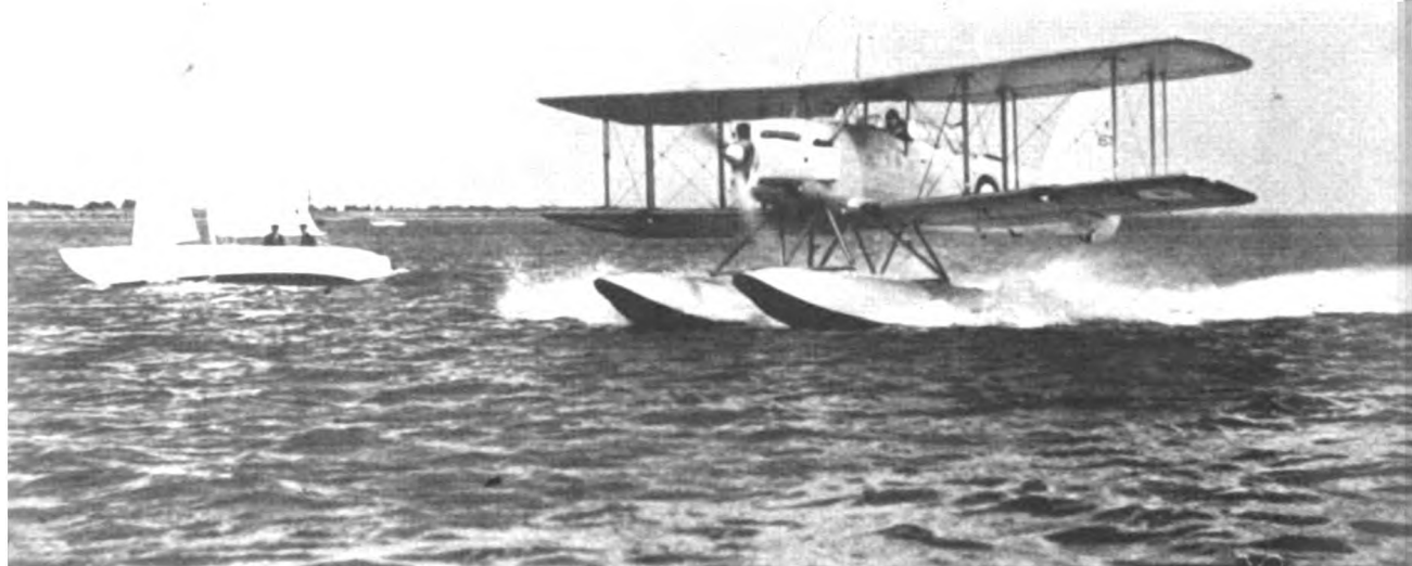
Built in 1936, the Fairey Seafox is for catapult duties. It is powered by a Napier Rapier engine of 355/370 h.p. and has a top speed of 124 m.p.h. The twin floats are of metal construction.
