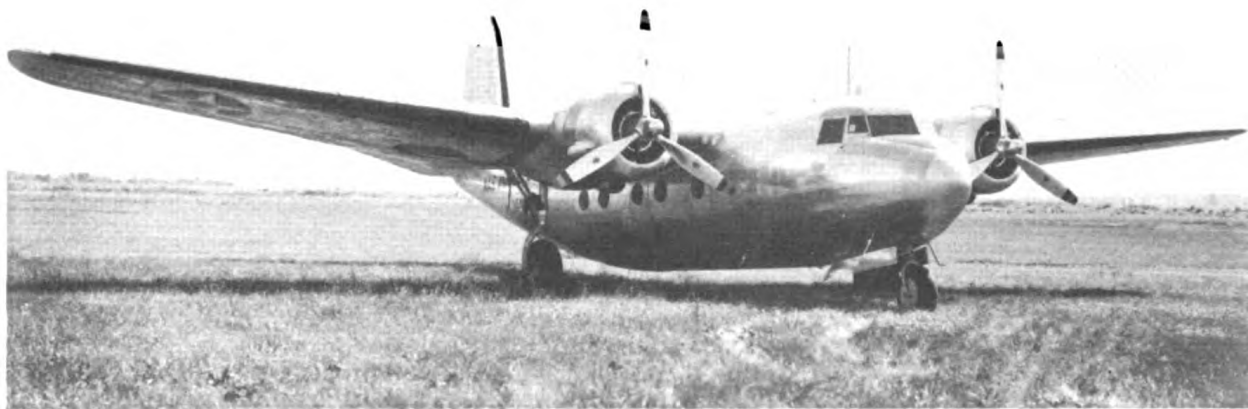
The Naval Air Service's Douglas R3D-1, like the C-42, is utilized as a cargo and personnel transport machine. It is a military version of the commercial DC-5 and maximum speed is 230 m.p.h.
